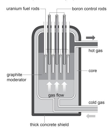
In a nuclear power station, a neutron is absorbed by a uranium nucleus, producing two lighter nuclei and more neutrons.
